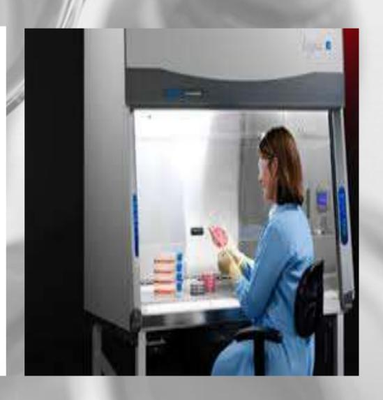
• The laminar flow hood provides an aseptic work area while allowing the containment of infectious splashes or aerosols generated by many
